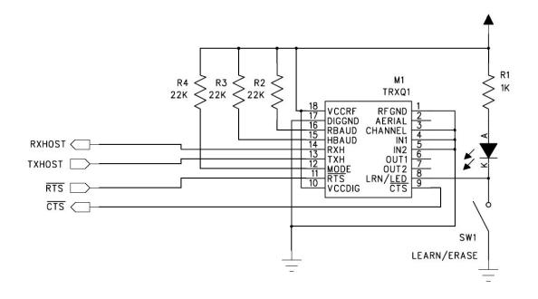
In some addressed mode applications the learn/erase components may not be required and the LRN/LED pin could be connected to the host micro controller which would be programmed to handle the functions of this pin.
